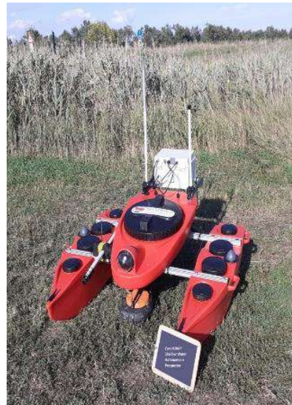
Fig.I.1.3a - Example of an autonomous vehicle. Open Swap Shallow Water Autonomous Prospector equipped with echo side scan sonar, single beam, and sub-bottom profiler.
