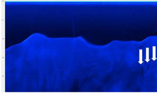
SSS 17 - Poles jutting out in correspondence with the layers relating to the river bank.
