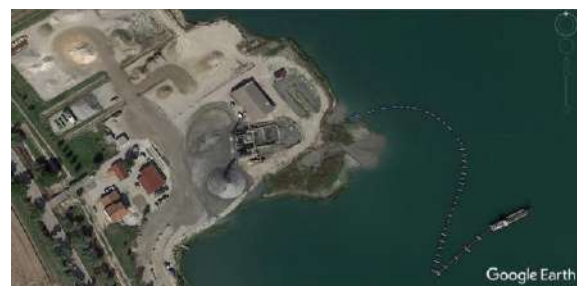
Fig.I.1.2 Example of the sand quarry, Cantoniera Cavallara, San Giovanni di Ostellato: working area and dredge system (Google Earth satellite image accessed (09/11/2023).
