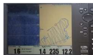
Fig.I.1.4c - Side-scan sonar operating according to the planned swaths: down image and track
