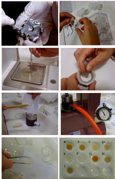
Fig.3. Initial steps in the preparation of the samples. a) Extraction b) Storage and Codification c) Manual crushing of the sample to homogenize and shrink the size of the grains, less than 2.0 μm. Pills Preparation. d) precision balance for weighing 2.5 mg of powdered sample and homogenization of the sample with KBr. Pressing the Pill. e) Introduction of the mixture into the mold. f) Mechanical press with the mold connected to a compressor, checking the pressure gauge that is 11 ton/cm 2 g) The process of drying of the tablets at a temperature of 110 ° C for subsequent analysis in the IR spectrometer.
