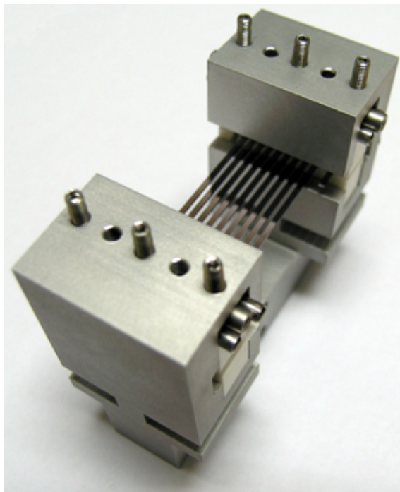
Figure 2. 29 A multi-strip crystal mounted in the holder.
