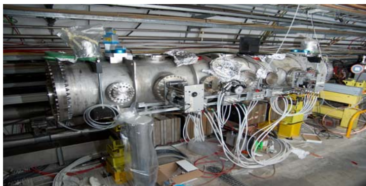
Figure 5.2 the UA9 tank with installed crystals and the tungsten scatterer
