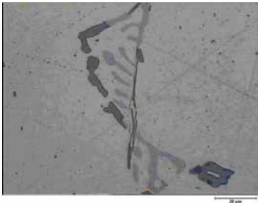
Fig. 7. Optical micrograph showing secondary phases particles.
