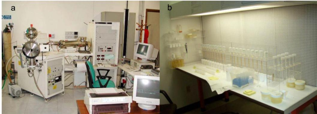
**Figure 1:** examples of a) the Thermal Ionization Mass Spectrometer (TIMS) ; b) the “clean room” similar to those used at IGG-CNR Laboratories of Pisa
