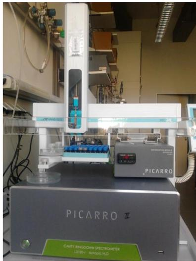
**Figure 2:** PICARRO L2120-i water isotope analyser at Helmholtz Centre for Environmental Research (UFZ) in Halle (Germany).
