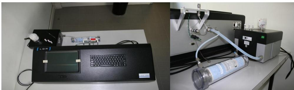
**Figure 3:** a) The Los Gatos CRDS LWIA 24-d liquid-water stable isotope instrument; b) vacuum pump, drierite column are shown in the background.
