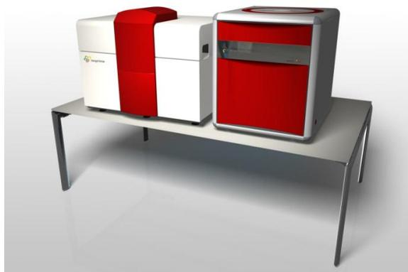
**Figure 11:** Elemental vario MICRO cube analyser and the IRMS Isoprime100 for the measurement of the elemental composition of carbon and nitrogen and relative isotopes ( $\delta^{13}\text{C}$  and  $\delta^{15}\text{N}$ )
